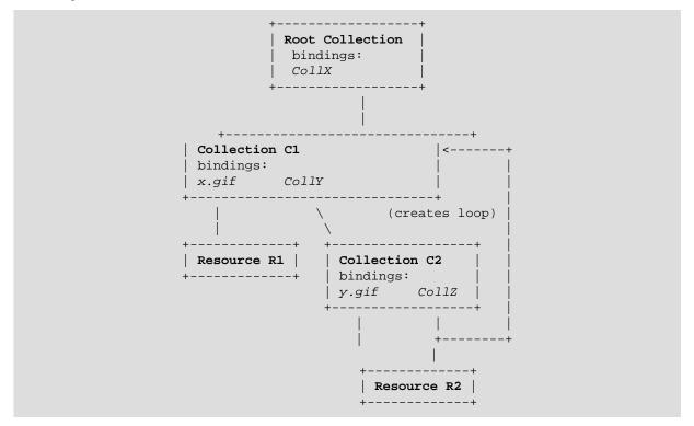
If a COPY request with "Depth: infinity" is submitted to /CollX, with a destination of /CollA, the outcome of the copy operation is that a copy of the tree is replicated to the target /CollA:
